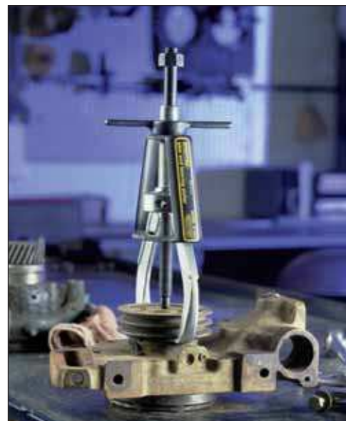
▲ EP-204 2 jaw puller positioned to pull a water pump.
