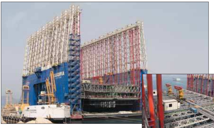
▼ PLC-controlled hydraulic movement: Enerpac stage -lift systems lift and lower the umbrella deck on the world's largest concrete block builder with 0,01 mm accuracy, provided by 30 hydraulic climbing units in an integrated hydraulic system.
