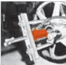
Combination of 50 ton capacity Push-Puller and cup pulling attachment simplifies the removal of a final drive axle seal.
