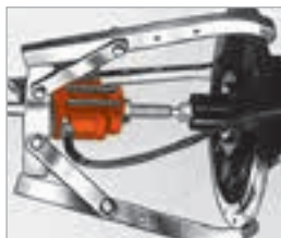
Combination of 50 ton capacity Push-Puller and cup pulling attachment simplifies the removal of a final drive axle seal.
