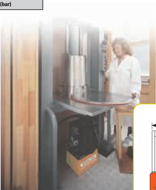
PE21 series pump and RD5513 cylinder used in a special press that produces pharmaceutical-grade extracts for herbal medicines.
