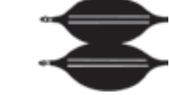
Stack up to two jacks together to increase effective lifting height.
