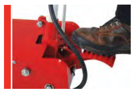
Foot pump for a fast lift to lift point*
